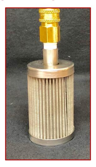
The **New Filter in Reservoir** for die lubrication systems is manufactured out of stainless steel and has a brass Quick Disconnect Coupling with an 1/8" NPT attached to the top for quick connection. This new filter is 1-1/2" in Diameter and 3" tall (4-1/4" including Quick Disconnect Coupling). The pleated filter screen is 100 mesh. Clean up is safe and easy by using soapy water.
